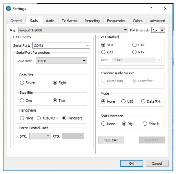
WSJT-X offers CAT (Computer Aided Transceiver) control of relevant features of most modern transceivers. To configure the program for your radio, select the **Radio** tab.
