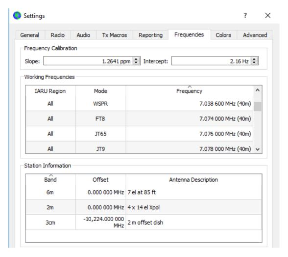
Working Frequencies: By default the **Working Frequencies** table contains a list of frequencies conventionally used for modes JT4, JT9, JT65, MSK144, WSPR, and Echo. Conventions may change with time or by user preference; you can modify the frequency table as desired.
