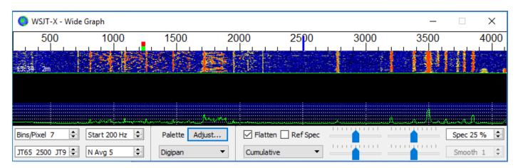
The position of the blue marker on the waterfall scale is set by the spinner control **JT65 nnnn JT9**, where nnnn is an audio frequency in Hz. In **JT9+JT65** mode the program will automatically decode JT9 signals only above this frequency. JT65 signals will be decoded over the full displayed frequency range.
